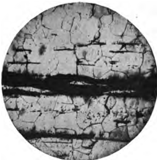
FIG. 195.—Wrought Iron. Longitudinal Section. Magnified 100 Diameters. (Boynton.)
